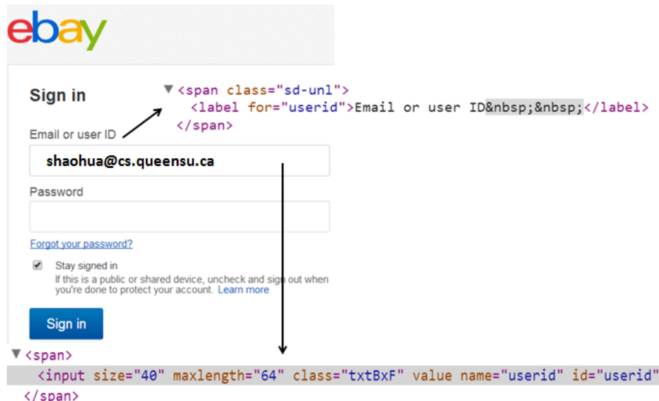
Fig. 3: A mapping between UI and its HTML coding.
