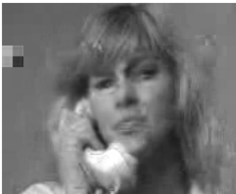
Figure 3.24: H.263 compressed Susie at 24 kbits/sec in average shadowed fading channel, 10 dB SNR, 15 kBd, 145 msec delay, showing frames 108, 120, 132, and 144 from top left to bottom right
