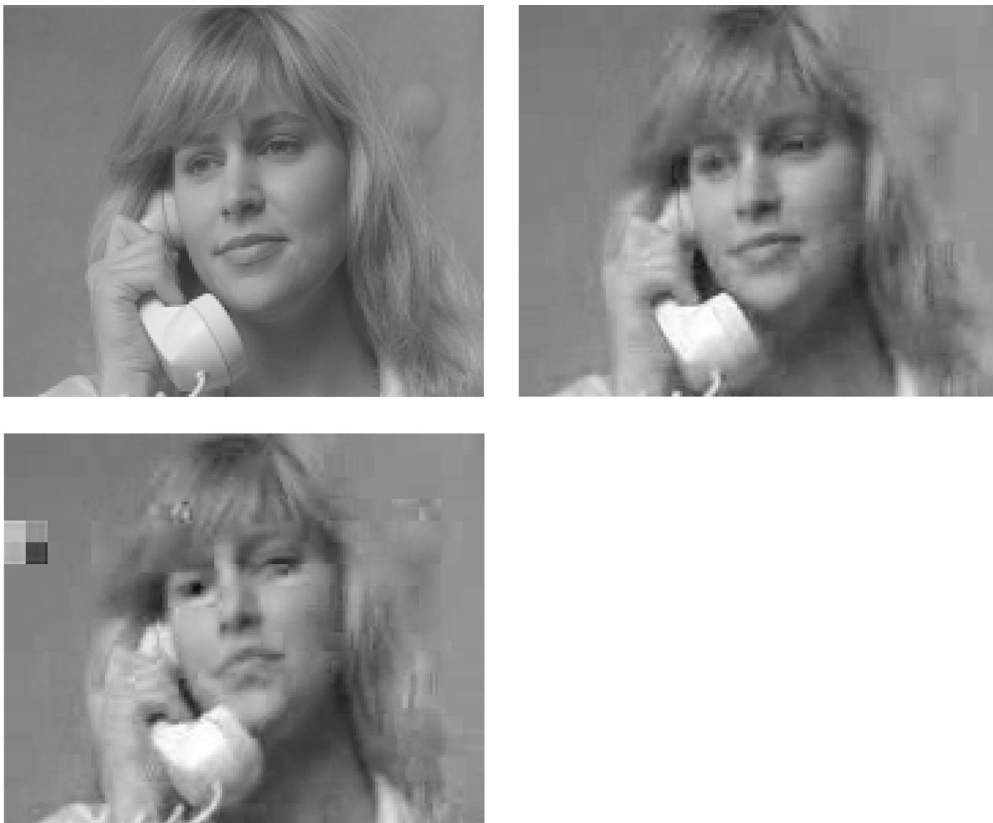
Fig. 7. Top-left: Original luminance frame 108 of Susie at 9.1 mbits/sec. Top-right: Susie at compressed 24 kbps in average shadowed fading channel at 12 dB SNR, 15 kbd, 145 ms delay channel. This top right image is visually indistinguishable from the case of an error-free channel. Bottom-left: worst-case channel distortion in 15 000 frames at 10 dB SNR, 15 kbd, 145 ms delay channel.
